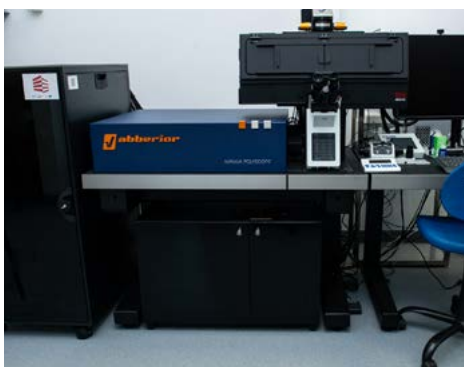
STED and 2D MINFLUX set-up at the Polish Advanced Light Microscopy Node, Nencki Institute in Warsaw.
